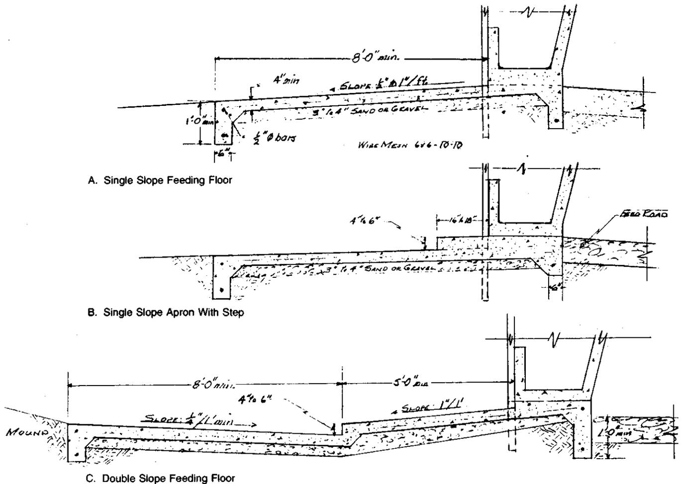
Figure 3. Typical Feeding Floor Sections
