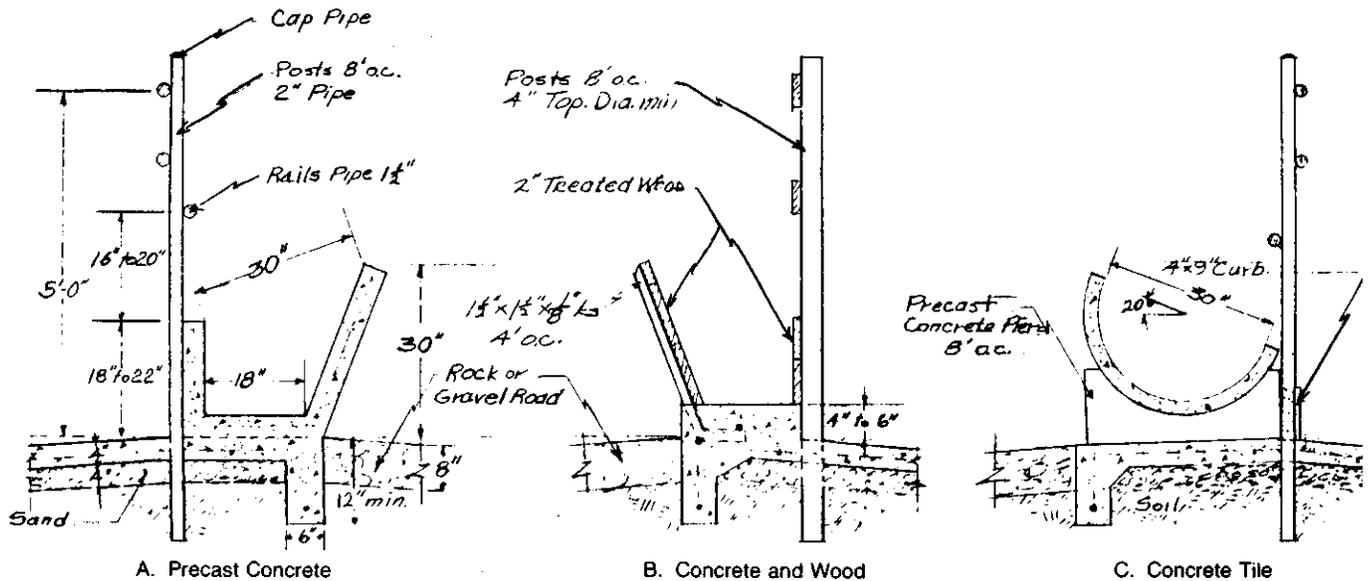
Figure 2. Typical Fenceline Feedbunk Sections.
