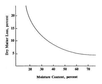
Fig. 1. Losses in Alfalfa as Influenced by Moisture Content when Raked.<sup>1</sup>
