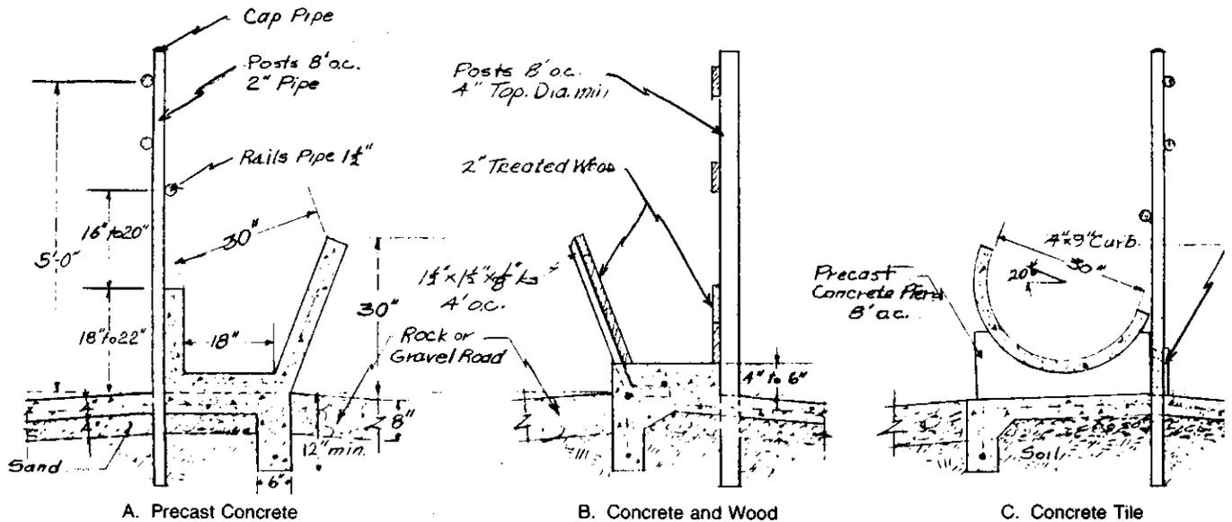
Figure 2. Typical Fenceline Feedbunk Sections.
