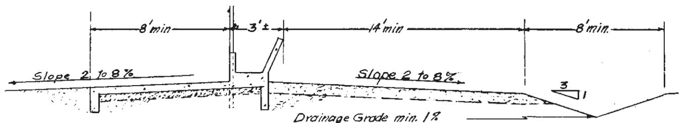
Figure 1. Feedbunk Grade and Drainage Section
